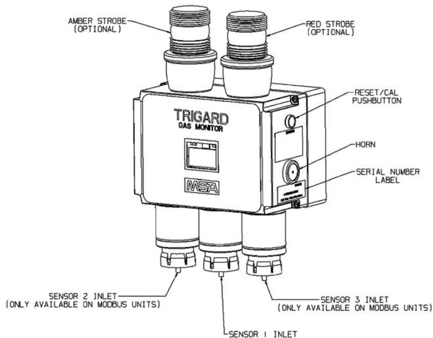
**Figure A-1. Trigard Gas Monitor with Additional Options**
