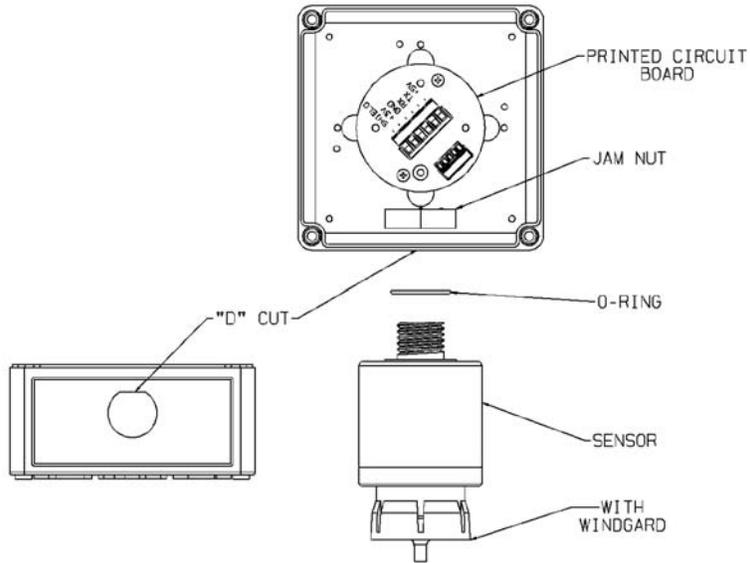
**Figure 1-5. General-Purpose Remote Sensor Assemblies**
