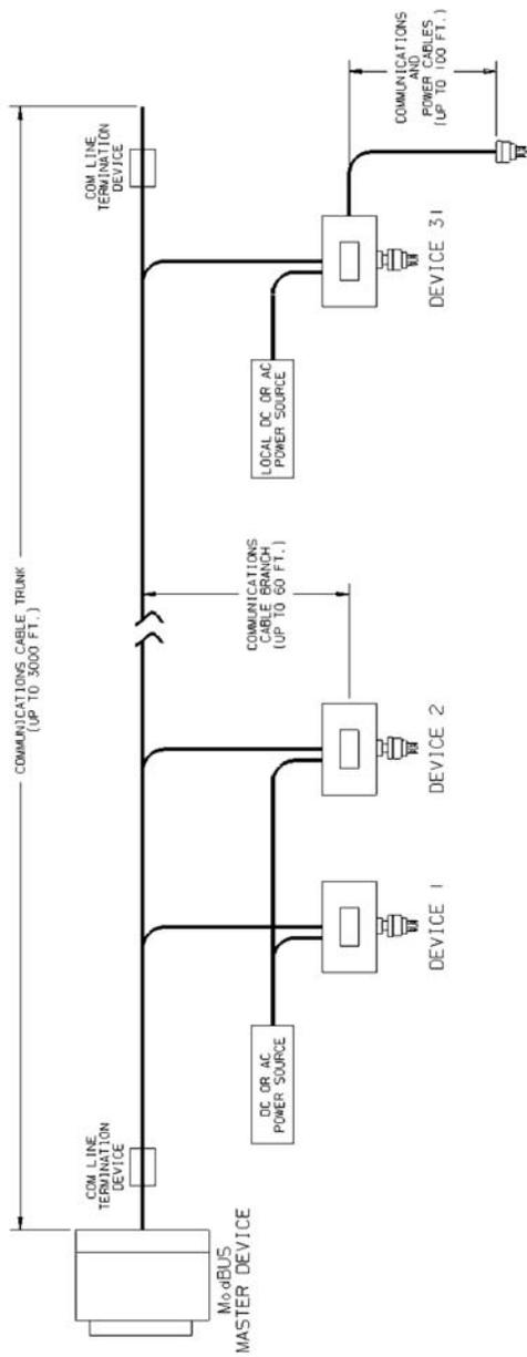
**Figure 3-1. Typical ModBUS Network Topography**
