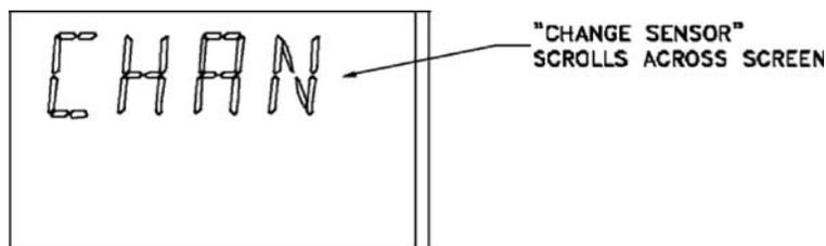
**Figure 6-1. "Change Sensor" Scrolls Across the Display**
