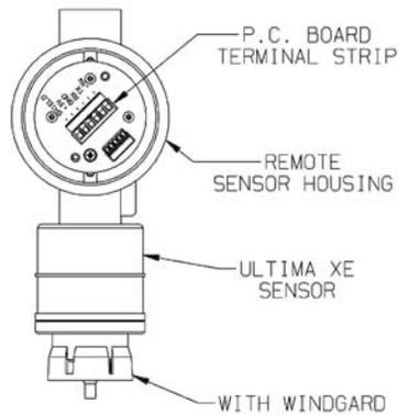
**Figure 1-6. Explosion-Proof Remote Sensor Assemblies**
