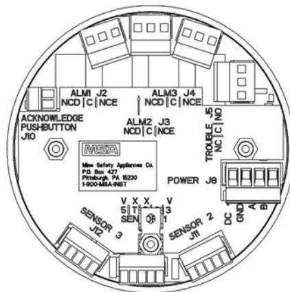
**Figure 3-5. ModBus PCB**
